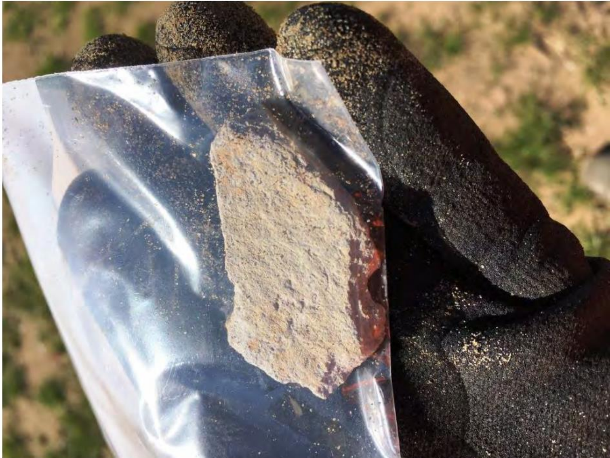
Figure 52: View of weathered-looking fibrous cement fragment found near Pit 1 (Source: Douglas Partners)
